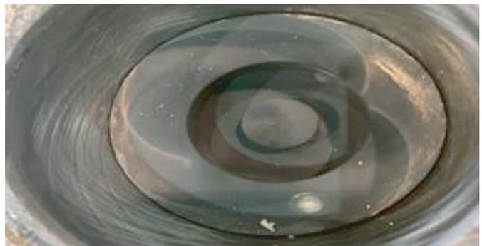
*The post-trials engine inspection identified no significant wear and no signs of cylinder glazing, no signs of damage due to changing of combustion timing related to the higher cetane number, and reduced soot deposition on the piston crowns, valves and injector nozzles*
