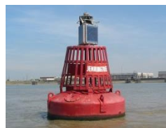
Solar panel on PLA buoy
