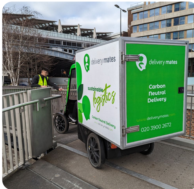
Figure 11. Tight Access at Blackfriars Pier. Showing the risk of contact with the handrail
